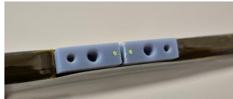
WLS fiber holders and SiPM mounts
