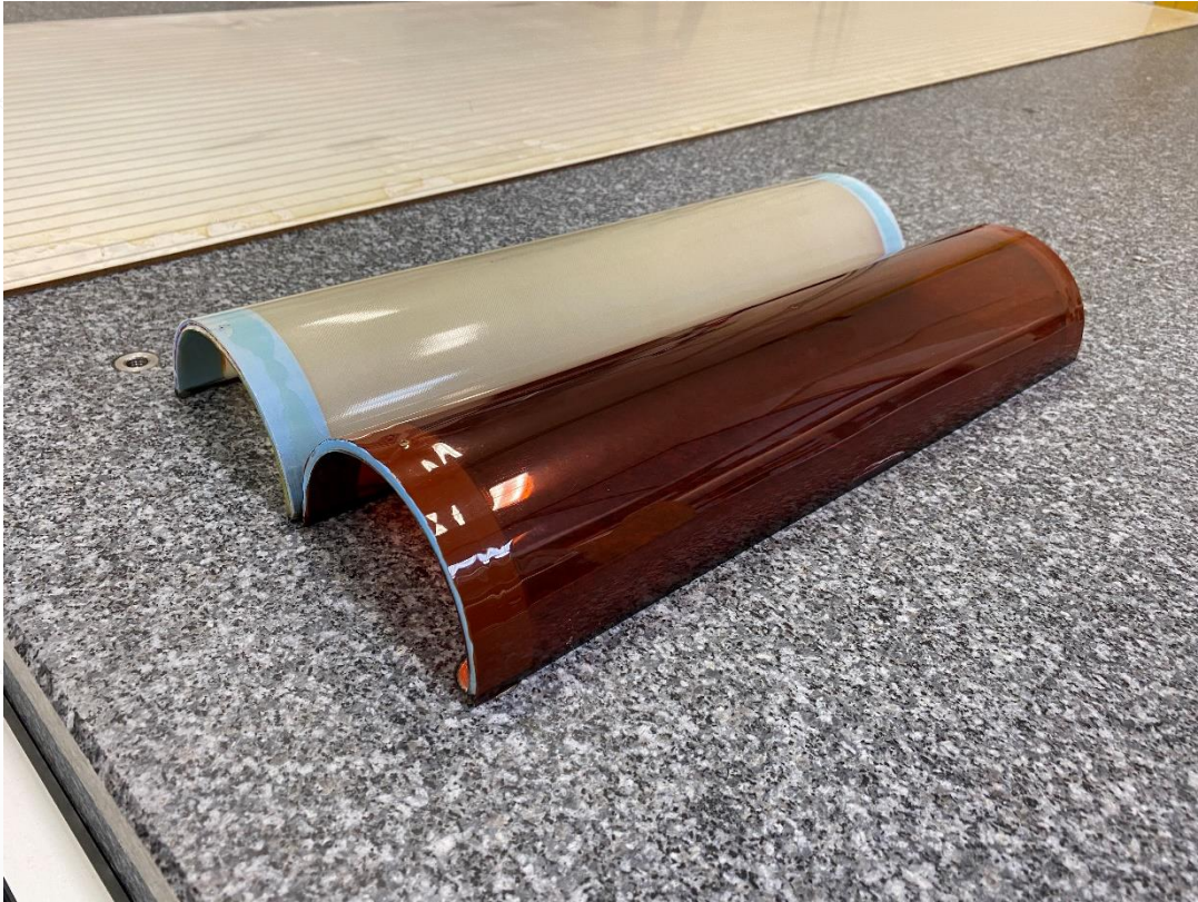
Second less rigid mechanical prototype. Material: Kapton (thickness = 200 microns)
