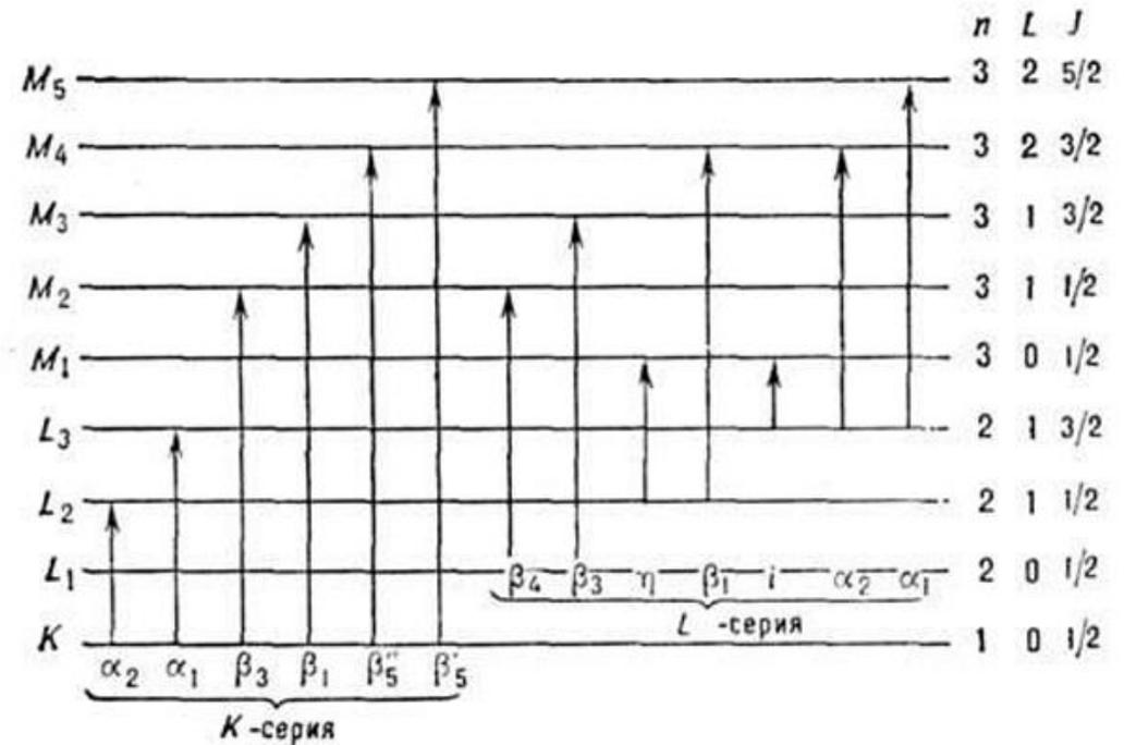
Pic 3: Diagram of the K-, L- and M-levels of atomic energy
