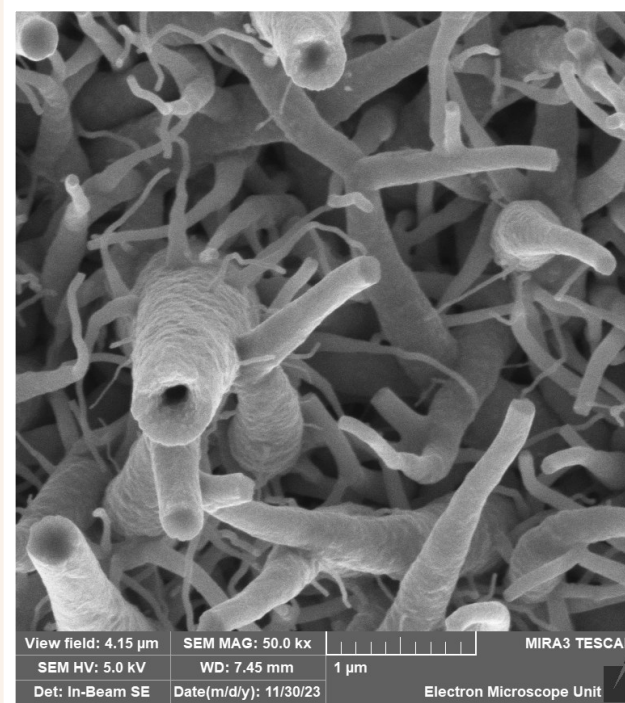
SEM image of CuS developed on copper substrate (Credit: A.S. Khameneh)
