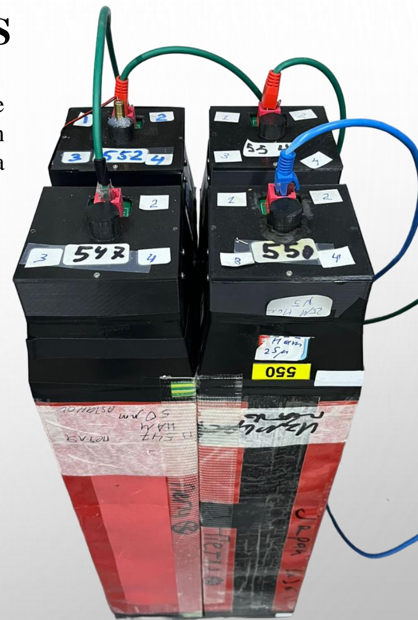
Fig. 13. Four calorimeter modules covered in light-isolation paper, connected to FERS
