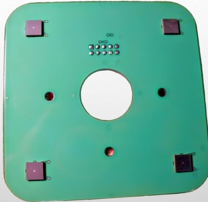
Fig. 12. Printed circuit board with 4 MPPC diodes
