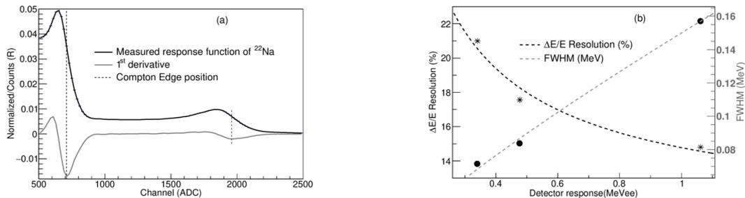
**Fig. 2.** a) The measured response functions of stilbene from the  $^{22}\text{Na}$  source and its calculated first derivative. b) The amplitude dependent resolution (FWHM) in the detector.
