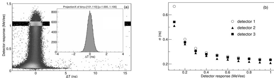
**Fig. 4.** a) The two-dimensional spectrum of time difference in both modules (detector 1 and 2) at the amplitude signal in detector 1 exceeds 1 MeVee. b) The dependence of time resolution on pulse amplitude for each detector in the energy range 0.1 - 1.0 MeVee.
