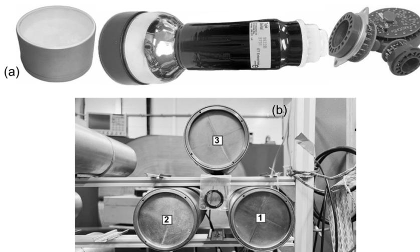
**Fig. 1.** a) A single detector module comprises a stilbene crystal, ET-Enterprise 9822B PMT and voltage divider. b) The configuration of the three detectors for time measurement with  $^{60}\text{Co}$  source.
