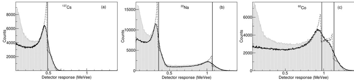
**Fig. 3.** The simulated and measured response functions of  $^{137}\text{Cs}$ ,  $^{22}\text{Na}$  and  $^{60}\text{Co}$   $\gamma$ -sources in the stilbene detector. The measured data is presented in hatch-filled histograms, while the GEANT4 calculation of energy deposited are shown with dash-lines and black lines shows the same but with instrumental energy resolution is taken into account. The vertical line represents the Compton edge positions defined with the first derivative method.
