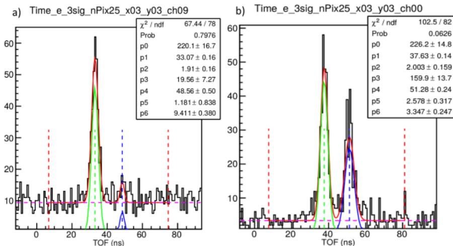
Time spectra. a)–time spectra obtained by detector # 10 far from tagged neutron beam, b)–time spectra obtained by detector # 1 placed on neutron's beam trajectory. Peak related to  $\gamma$ -quanta fitted by green curve,  $n$ -peak fitted by the blue curve.
