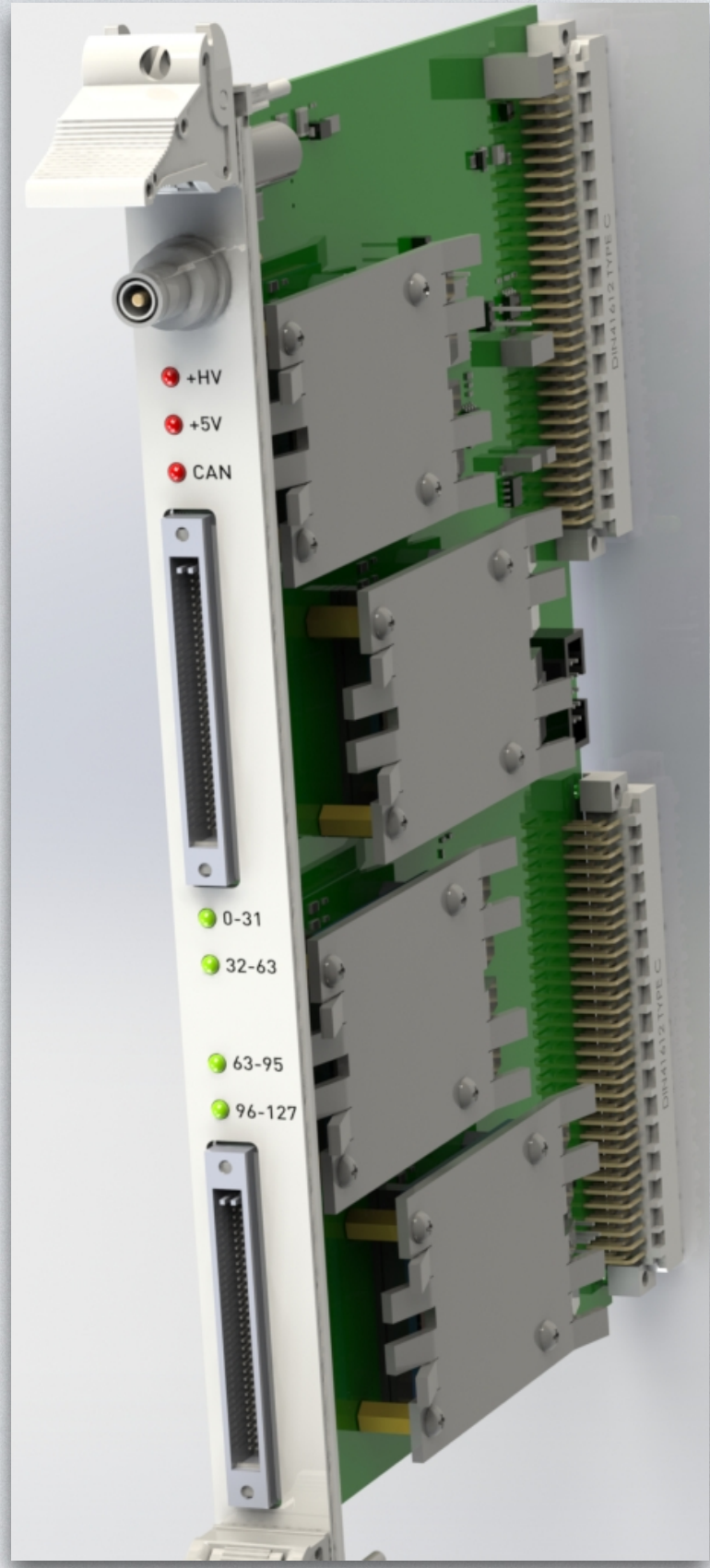
128 channel power supply unit VME 6U PCB unit
