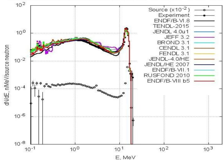
The neutron leakage spectrum from a Mn sphere (D=60 cm) with  $^3\text{H}(d,n)^4\text{He}$  neutron
