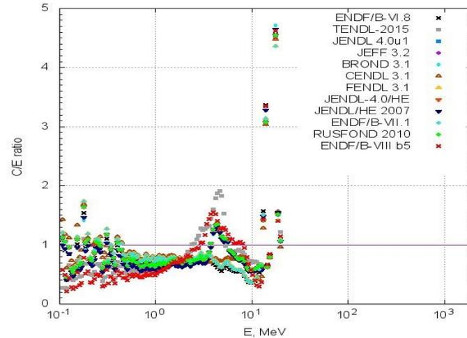
The neutron leakage spectrum from a Si sphere (D=60 cm) with  $^3\text{H}(d,n)^4\text{He}$  neutr
