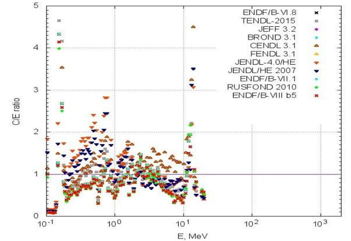
The neutron leakage spectrum from a Zr sphere (D=60 cm) with  $^3\text{H}(d,n)^4\text{He}$  neutr
