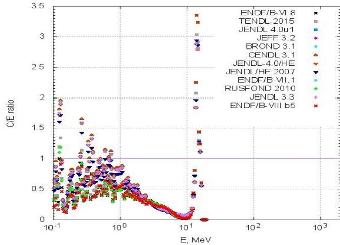
The neutron leakage spectrum from a Co sphere (D=40 cm) with  $^3\text{H}(d,n)^4\text{He}$  neutr
