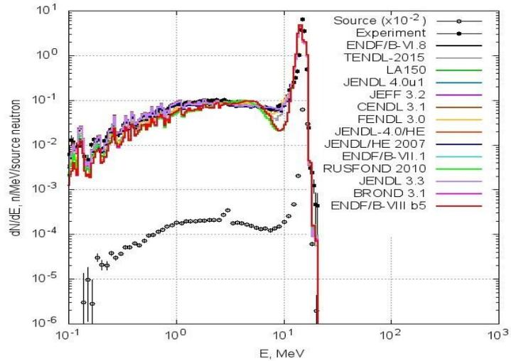
The neutron leakage spectrum from a Co sphere (D=40 cm) with  $^3\text{H}(d,n)^4\text{He}$  neutron
