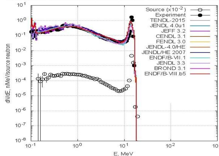
The neutron leakage spectrum from a W sphere (D=40 cm) with  $^3\text{H}(d,n)^4\text{He}$  neutron
