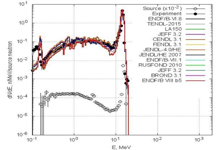
The neutron leakage spectrum from a Zr sphere (D=60 cm) with  $^3\text{H}(d,n)^4\text{He}$  neutron
