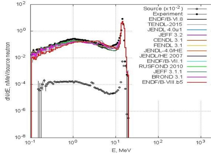
The neutron leakage spectrum from a Si sphere (D=60 cm) with  $^3\text{H}(d,n)^4\text{He}$  neutron
