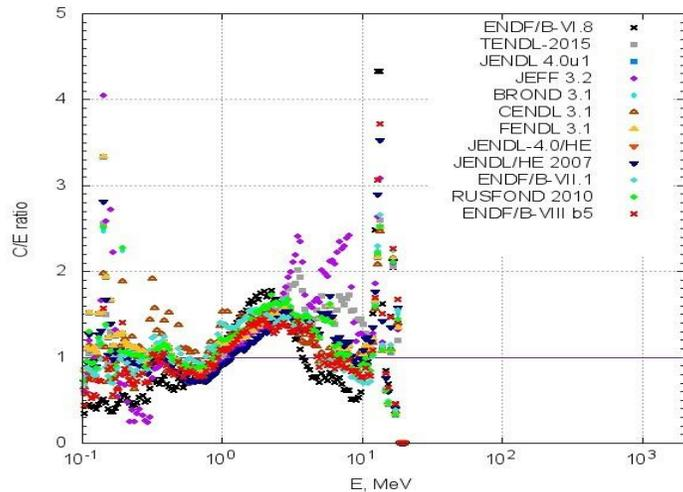
The neutron leakage spectrum from a Mn sphere (D=60 cm) with  $^3\text{H}(d,n)^4\text{He}$  neutr
