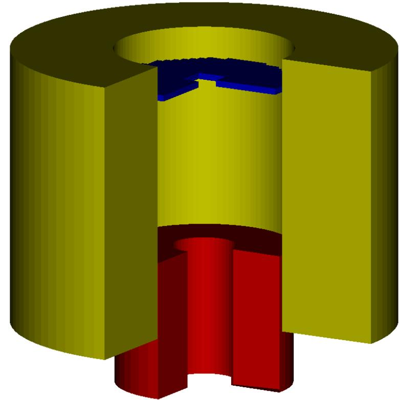
Solid-state 3D model of calorimeter E391a for KEK
