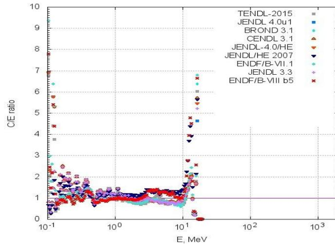
The neutron leakage spectrum from a W sphere (D=40 cm) with  $^3\text{H}(d,n)^4\text{He}$  neutr
