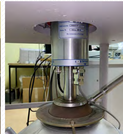
Spectrometer of gamma radiation SEG-1KP-IFTP (detection unit BDEG-OGK-3K)
