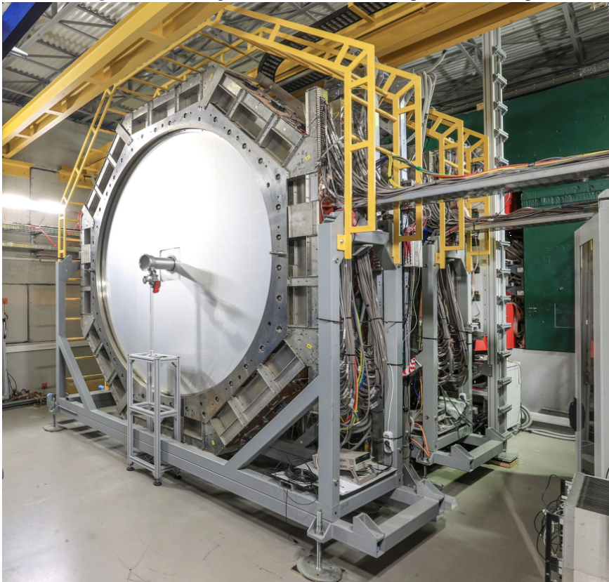
Fig. 25. DCH integrated into the BM@N experimental setup.
