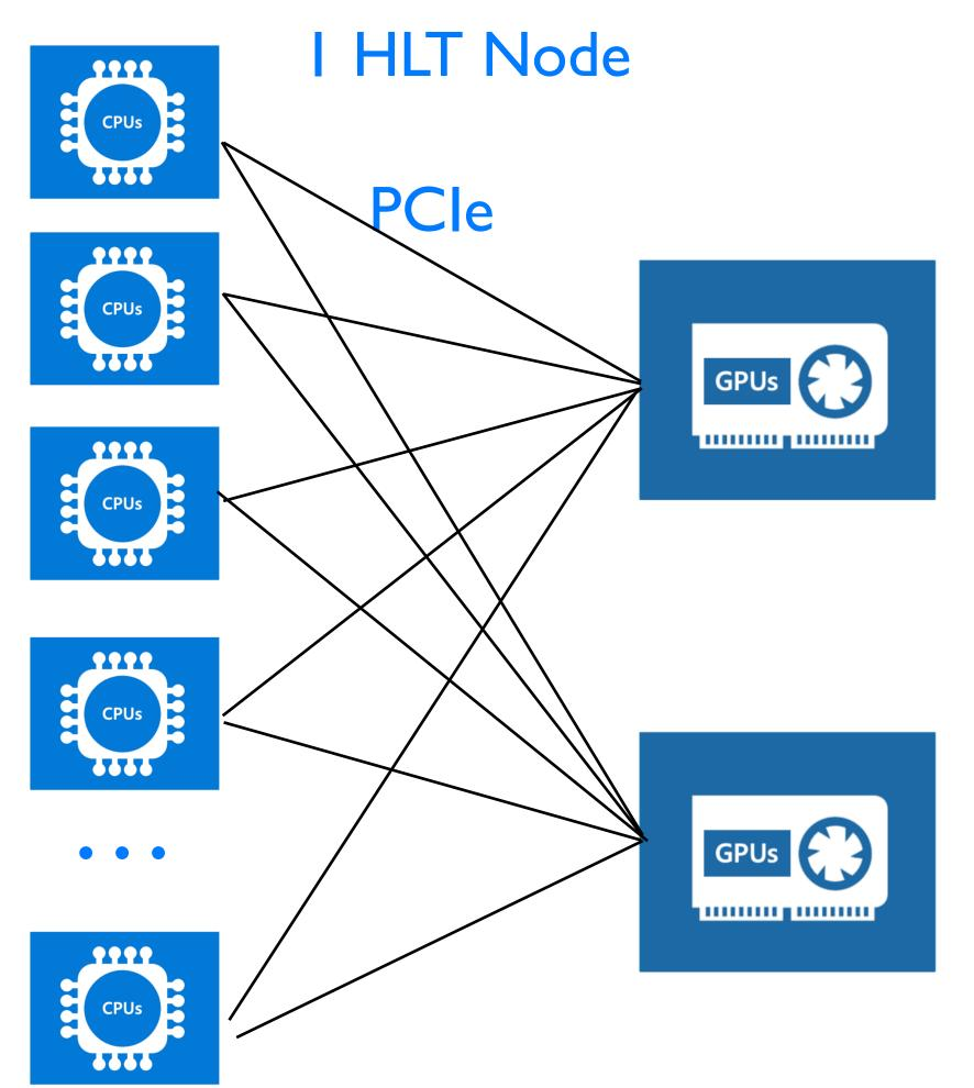
2 AMD EPYC 7763 CPUs(2x64 physical cores;2x64x2 hyperthreads)
