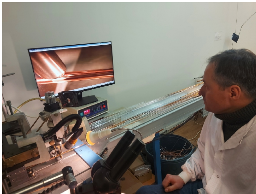
Figure 9.6: The straw production setup with an ultrasound head with movable fixation at the frame.
