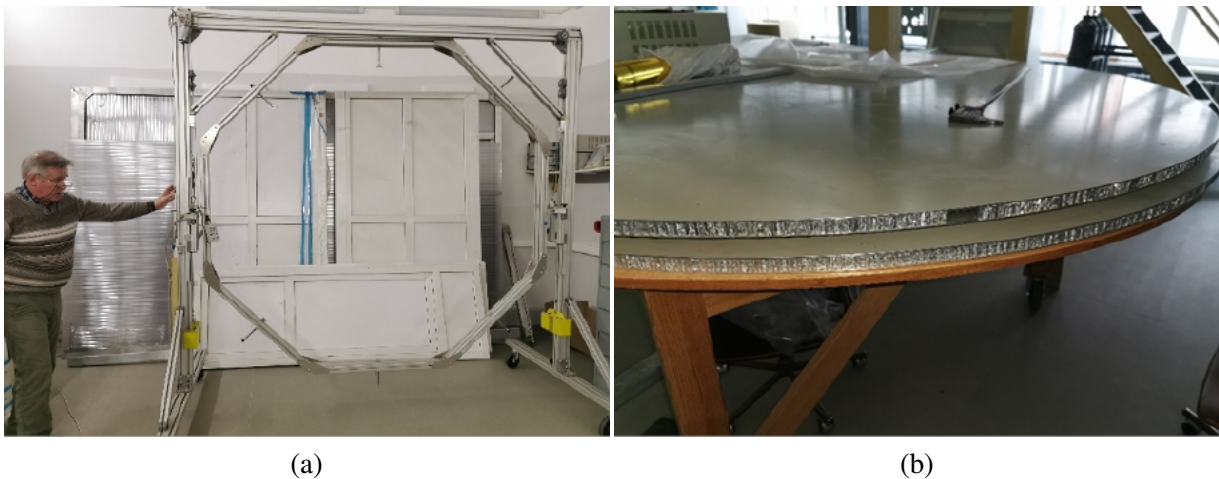
Figure 9.41: (a) Technological equipment for assembly. (b) Octagonal rotary platform and a portable honeycomb board for assembling are shown. The diameter of the portable board is 2300 mm, and the thickness is 50 mm.
