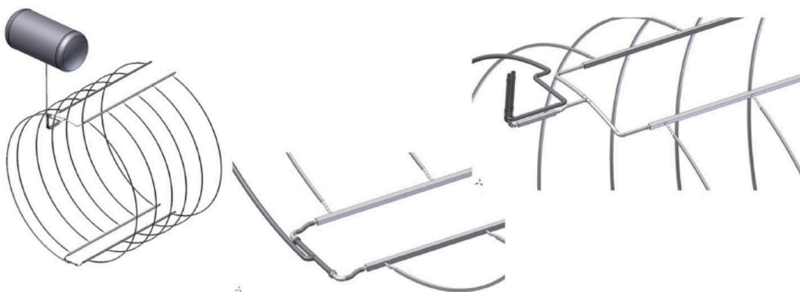
Figure 5.17: Thermosyphon circuit of the SPD solenoid showing the two-halves assembly of the cold mass, as well as the height of the chimney and position of the control dewar.
