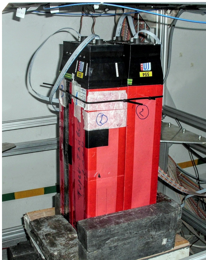
Figure 4.21: Photo of the calorimeter test setup consisting of 4 modules of the size 11 \times 11 \text{ cm}^2 , with the total cross-section of 22 \times 22 \text{ cm}^2 .
