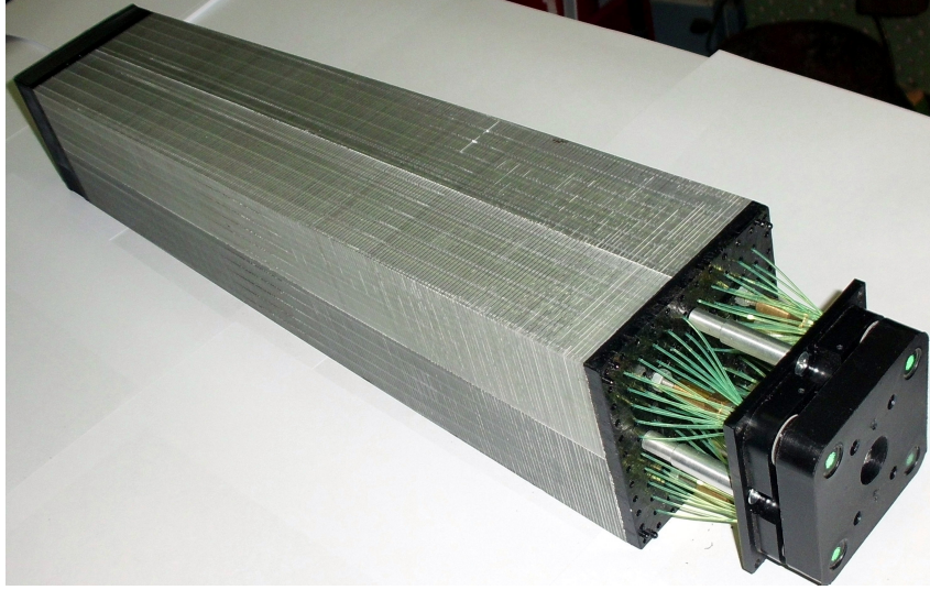
Figure 4.18: Photo of a single module consisting of 4 cells with 220 layers of the scintillator and the absorber with a thickness of 1.5 mm and 0.3 mm, respectively. Four bundles of fibers for guiding the light to the multi-pixel photon counters (MPPC) can be seen.
