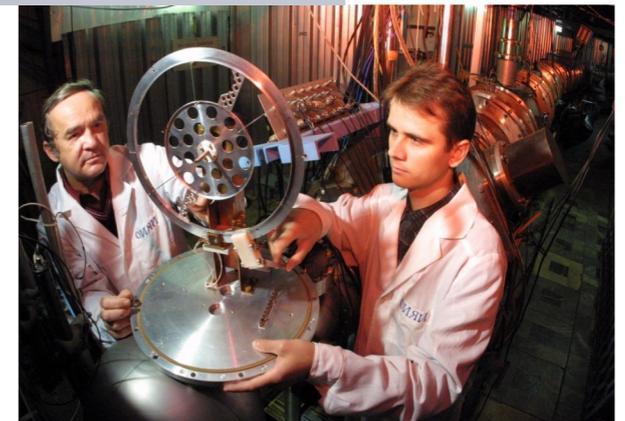
Deuterons and protons in coincidences using scintillation counters
