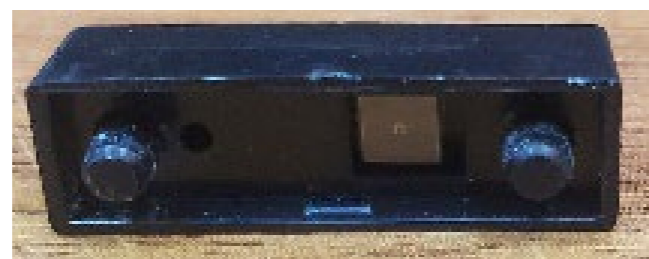
Sketch of the strip with SiPM board and housing. The real look of the SiPM PCB inserted to the housing
