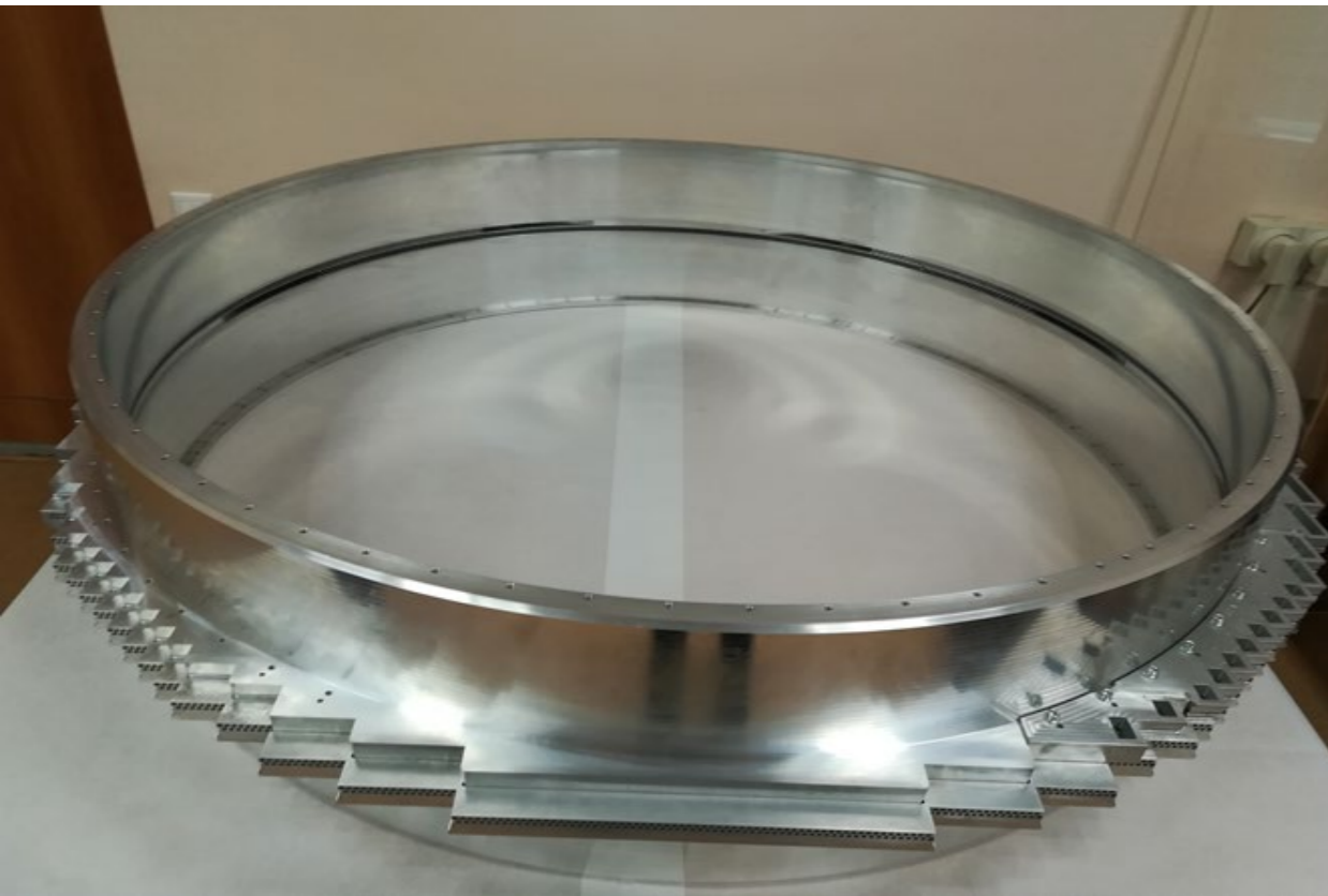
Support frame of the straw module
