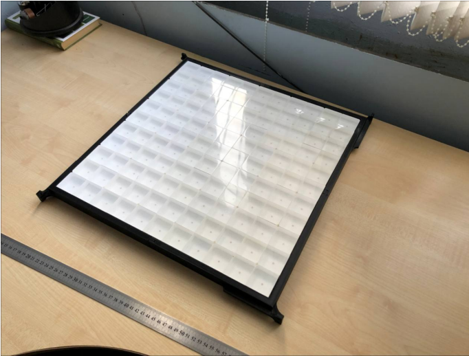
scintillator layer assembled
