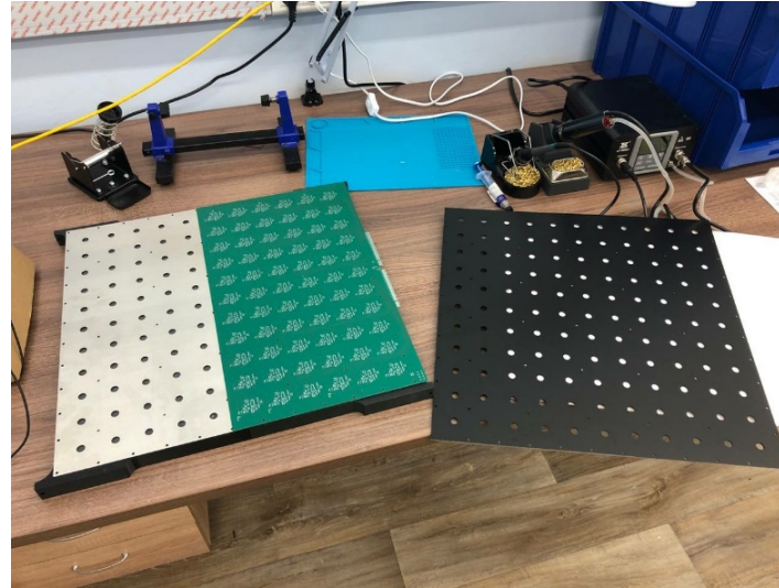
active layer PCB positioning
