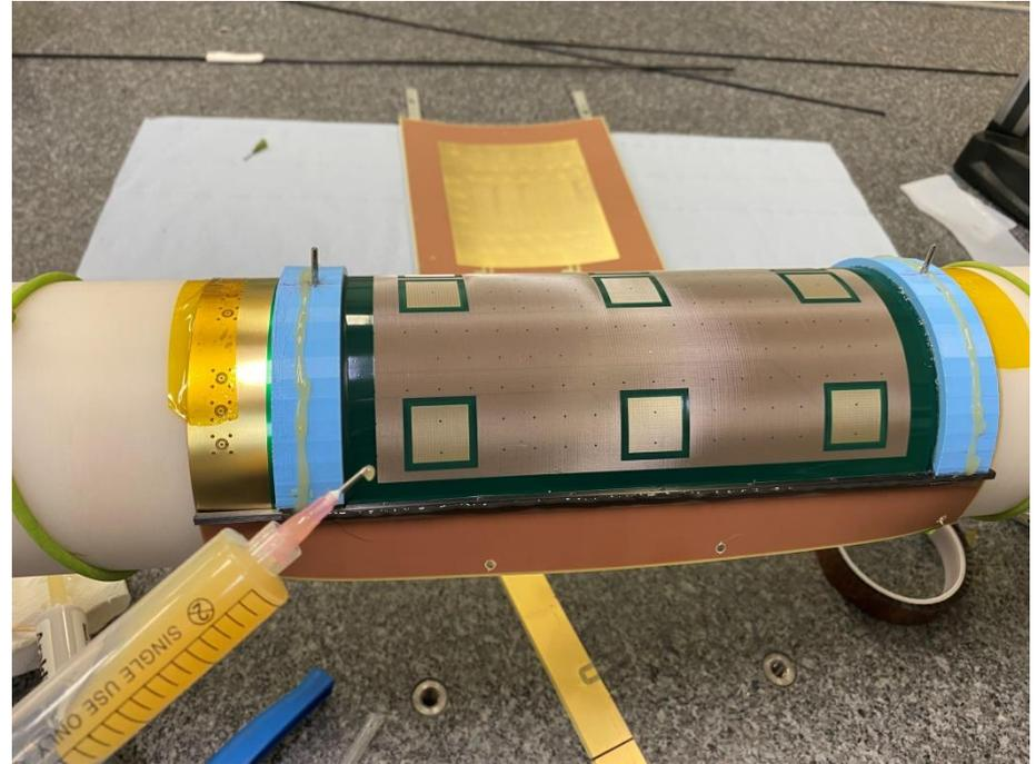
Signal electrodes shaped as 9 pad to check gain ( $\Leftrightarrow$  gap) uniformity after bending
