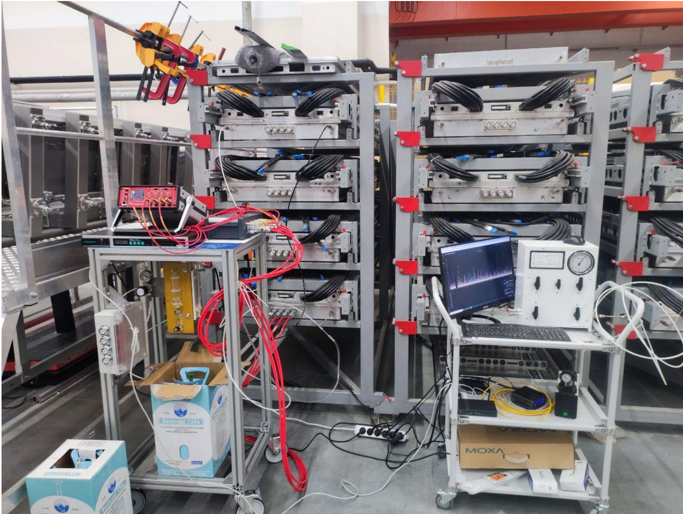
HV and leakage test of stored modules
