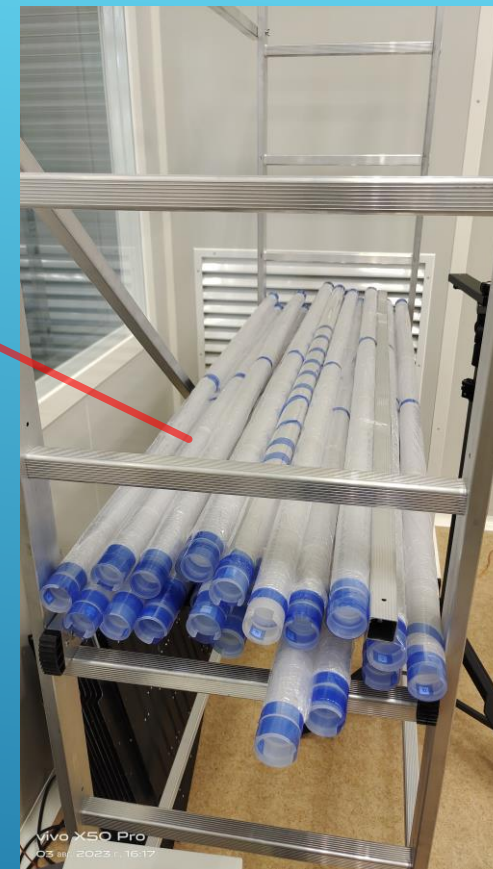
Rods D=40 mm – ready for installation
