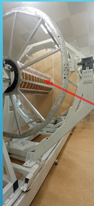
Both flanges and HV electrode: alignment to do and all elements glued to C1-C2 - 11/07/2023
