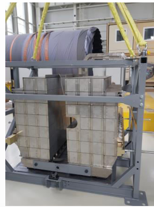
FHCAL assembled on the platform is ready to be installed in the Pole.
