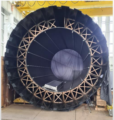
Carbon fiber support frame delivered and unpacked, sagita ~ 5 mm at full load
