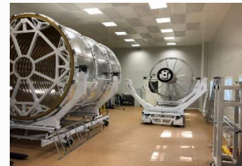
TPC cylinders, central membrane, service wheels, readout chambers, gas system - ready - final vessel assembly by the end of year
