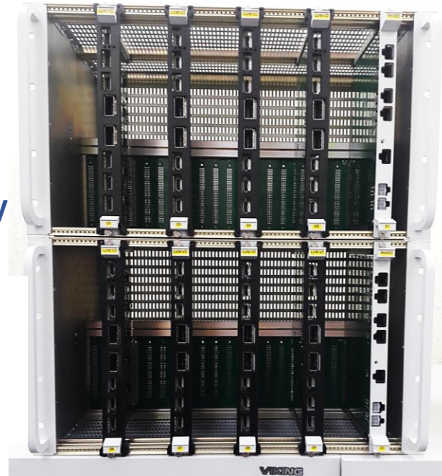
Crates with Fan-out & LV modules
