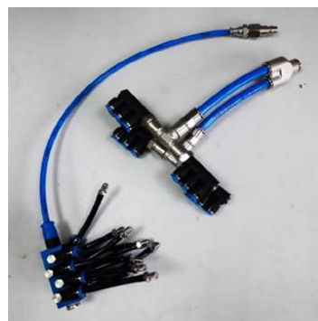
Cables and distributors of air flow to FFD modules
