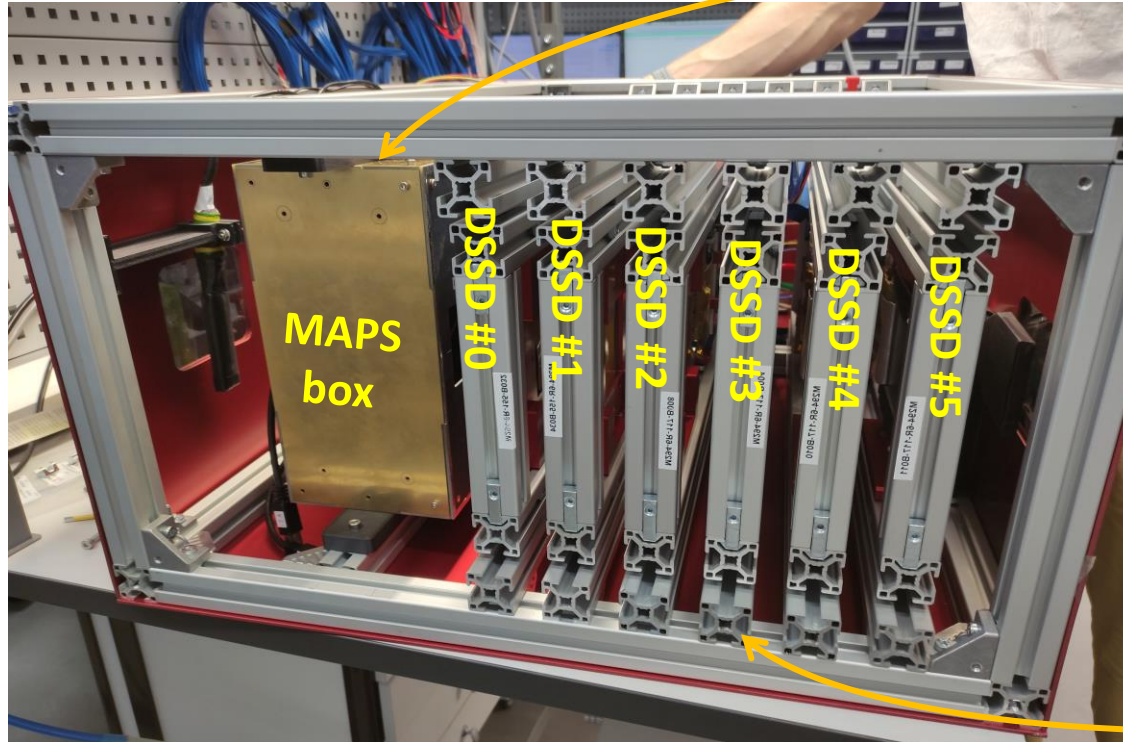
Beam telescope with 3 layers of MAPS & 6 layers of DSSD sensors
