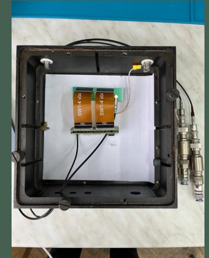
Cast iron case with FEC connected by flexible PCB to PCB with Ccal
