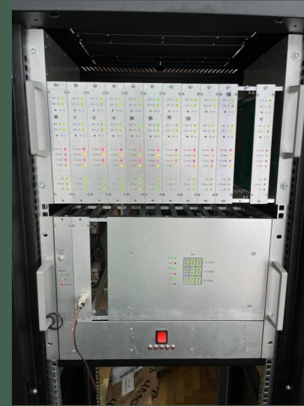
Front and back side of 1 Gate crate, in top-12 Gate modules, in bottom PSU
