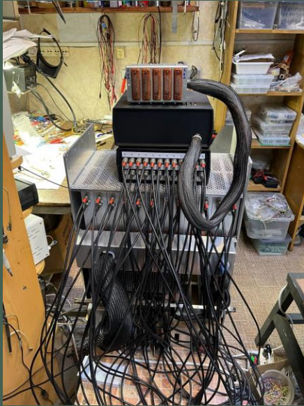
Front and back side of Gate with connected devices for testing PSU and 12 Gate modules simultaneously
