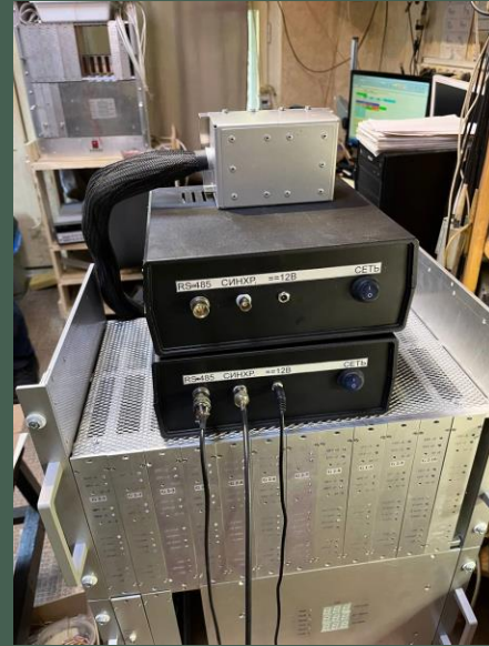
Front and back side of Gate with connected devices for testing PSU and 12 Gate modules simultaneously
