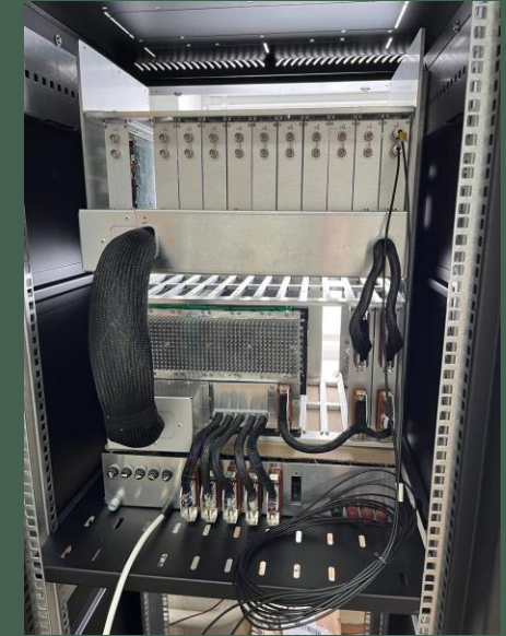
Front and back side of 1 Gate crate, in top-12 Gate modules, in bottom PSU
