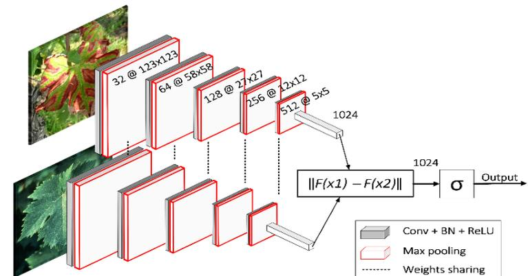
Our best siamese convolutional architecture. «Conv» means the convolutional operation, «BN» is a batch normalization, «32 @ 123x123» – 32 filters with the particular size
