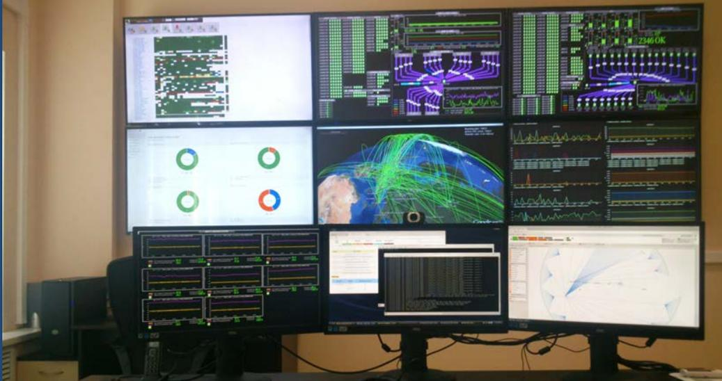
The system allows one, in a real time mode, to observe the whole computing complex state and send the system alerts to users via e-mail, sms, etc. ~ 850 elements are under observation ~ 8000 checks in real time ~ 100 scripts
