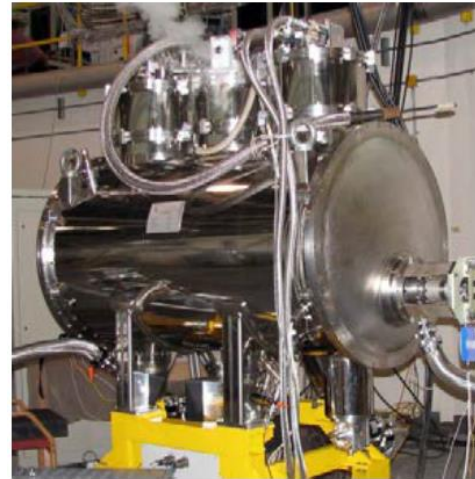
27-pole 4.2 Tesla, \lambda=48 mm superconducting wiggler for Canadian Light source. 2007
