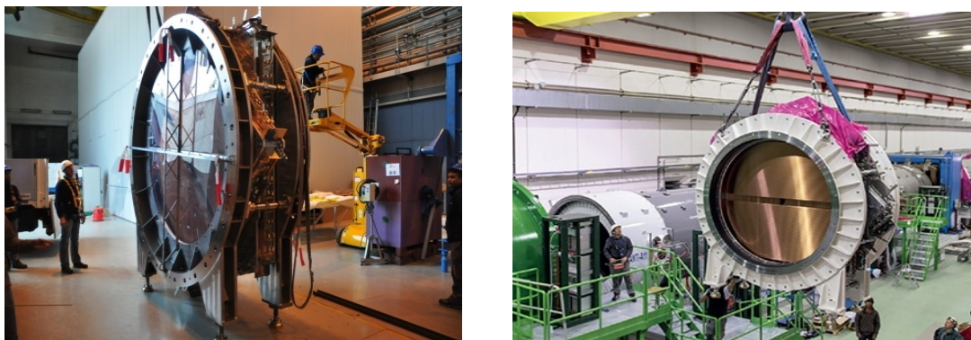
Figure 2. A straw chamber assembled from 2 modules (left) and its installation in the NA62 experimental setup (right).
