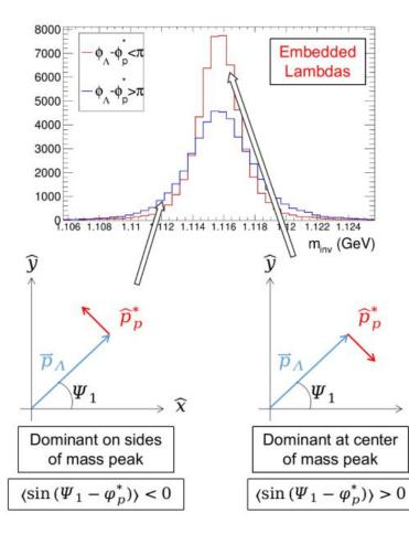
This method can deal with tracks crossing: daughter particles tracks with opposite charges are bended in the opposite directions in the magnetic field, and these tracks may cross each other -> creates 2 peaks distribution. Solution: fit Sig with 2 gausses
