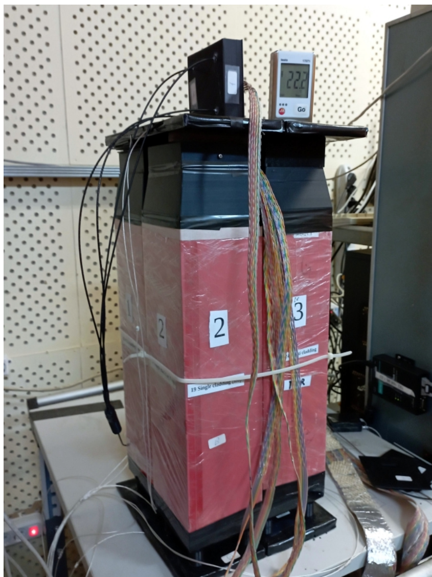
Figure 6.13: Photo of the calorimeter test setup consisting of 4 modules of the size 11 \times 11 \text{ cm}^2 , with the total cross-section of 22 \times 22 \text{ cm}^2 . The environment temperature was measured by thermistors, provided for each of the 4 MPPC boards, and by a digital thermometer as well. One of the boards in the light protection cover and the digital thermometer were placed on top of the setup. The optical fibers (visible in this photo) distributed the light from the LED generator.
