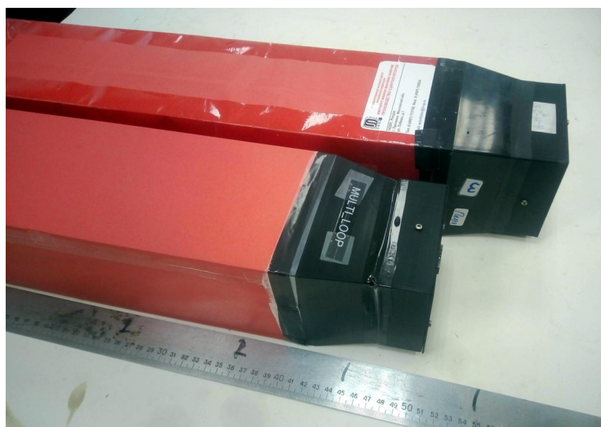
Figure 6.7: Two calorimeter modules covered in light isolation paper are shown in this photo. The modules have different lengths due to a different number of layers (190 and 220) and a different absorber thickness of 0.5 and 0.3 mm, respectively.
