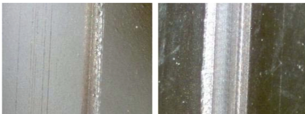
Figure 9.5: Quality of the welding seams of 0.4 mm (left) and 0.85 mm (right) at \times 60 magnification.
