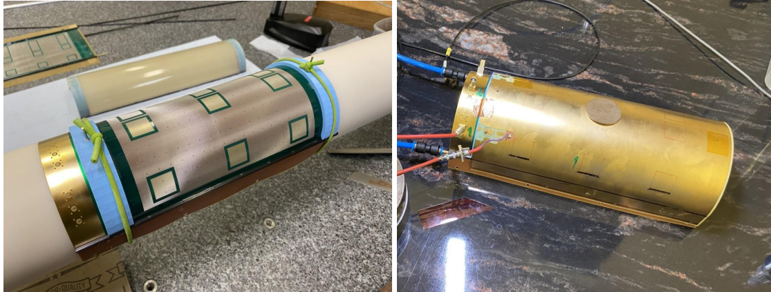
Figure 12.19: First cylindrical MM prototype. Left: assembling procedure. Bulk MM module bending and fixation on a template for gluing. Right: assembled module prepared for the very first functionality test.
