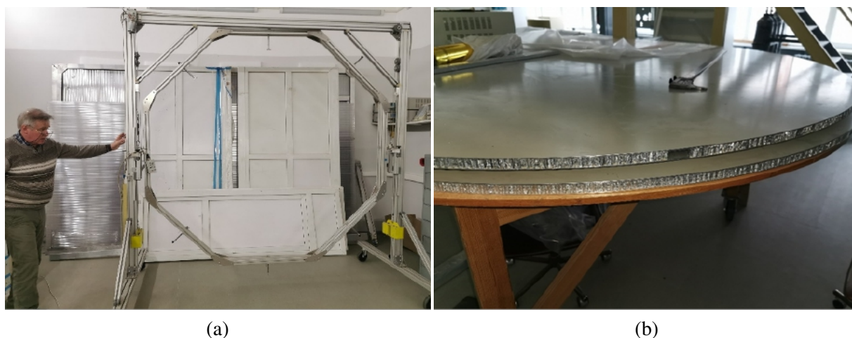
Figure 9.41: (a) Technological equipment for assembly. (b) Octagonal rotary platform and a portable honeycomb board for assembling are shown. The diameter of the portable board is 2300 mm, and the thickness is 50 mm.
