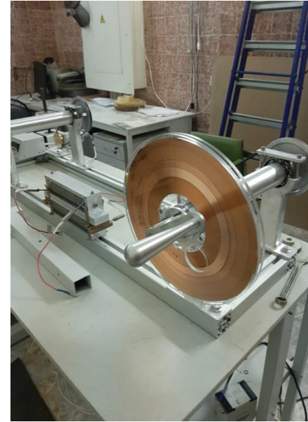
Machine for rewinding tape from reel to reel, 4 mm wide Tape from c-innovation on the reel
