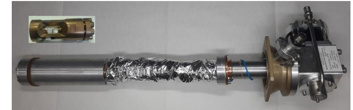
Fig.3 Cryostat-insert, temperature 3.6 -150 K and press on 10 GPa
