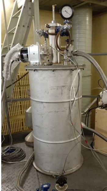
Fig.1 the photograph of a cryostat
