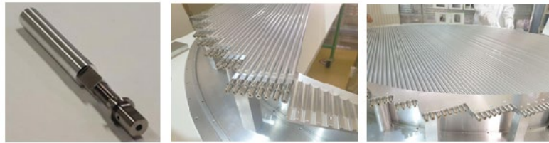
Fig. 22. Assembly of a tracker station for Phase-I
