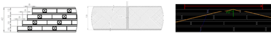
Fig. 45. Module pattern, technological gaps. Illustration of the muon track from -75 to 75 degrees of inclination and from -40 to +40 mm away from the central upper strip
