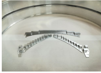
Fig. 27. Gas distribution block
