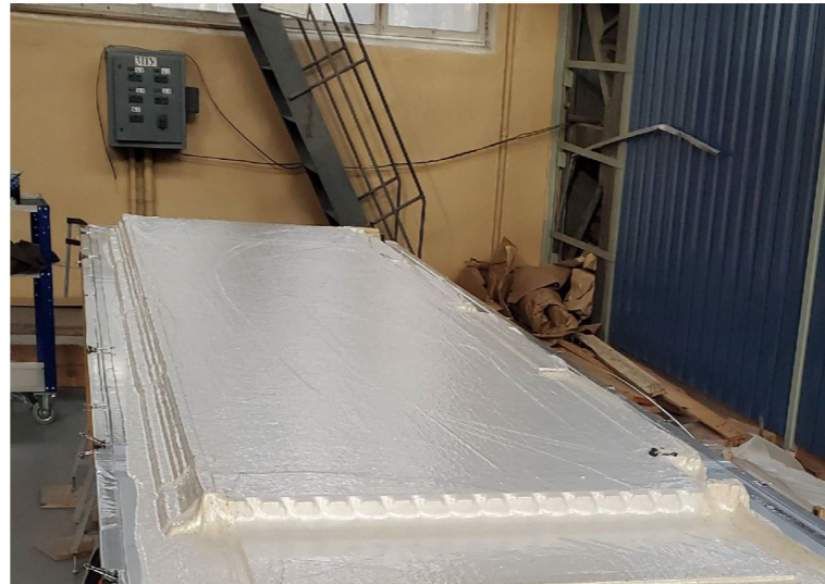
Compressed by 1 bar CRV module
