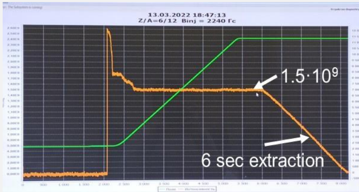
Magnetic field cycle and carbon beam intensity in the Nuclotron
