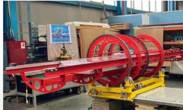
TOF module in the carbon fiber mainframe
