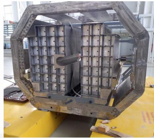
FHCAL assembled on the platform, ready to be installed in the Pole (modules are equipped with FEE)
