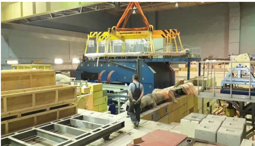
The coil sections move in cyclotron hall
