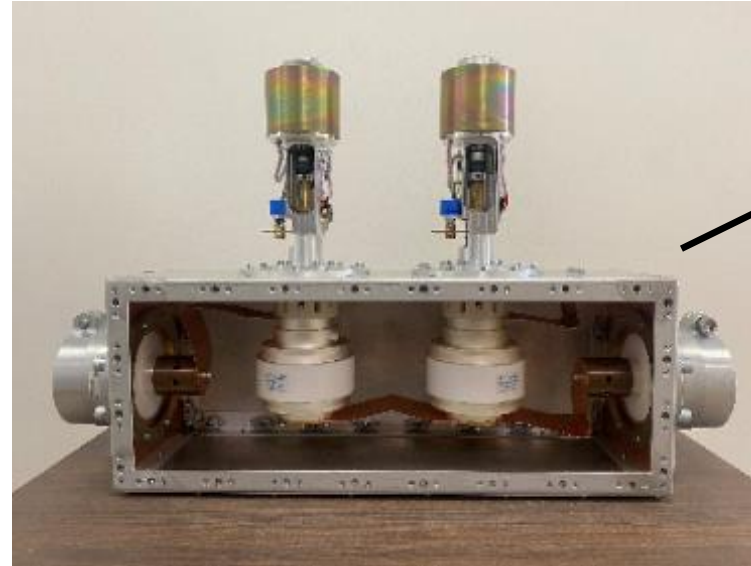
Load matching system (matching the load to the of the feeder line)
