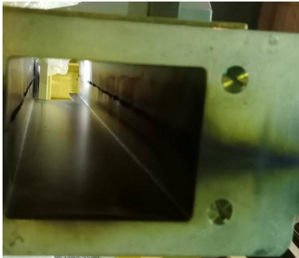
Traces from the beam on the magnetic channel MK2 (before modernization)
