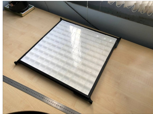
scintillator layer assembled
