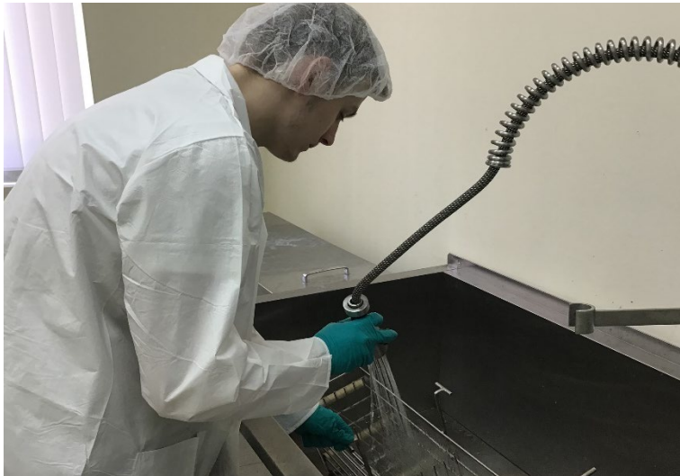
Glass cleaning with ultrasonic wave & deionized water
