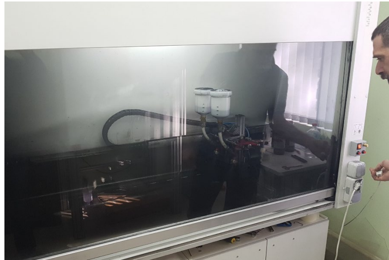
Automatic painting the conductive layer on glass
