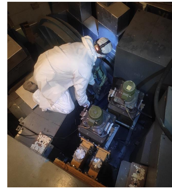
Pic. 3, 4. Replacing the grease of the bearings of the background HRFD chopper.
