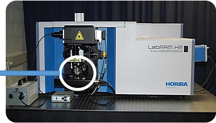
Raman spectrometer LabRam, by Horiba
