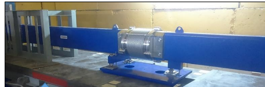
Focusing part of neutron guide
