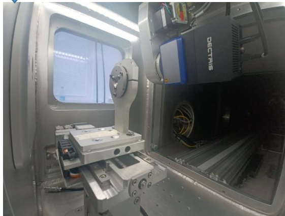
DAC in an X-ray beam. pressure up to 100 Gpa.
