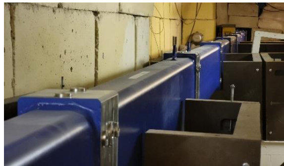
Curved part of neutron guide
