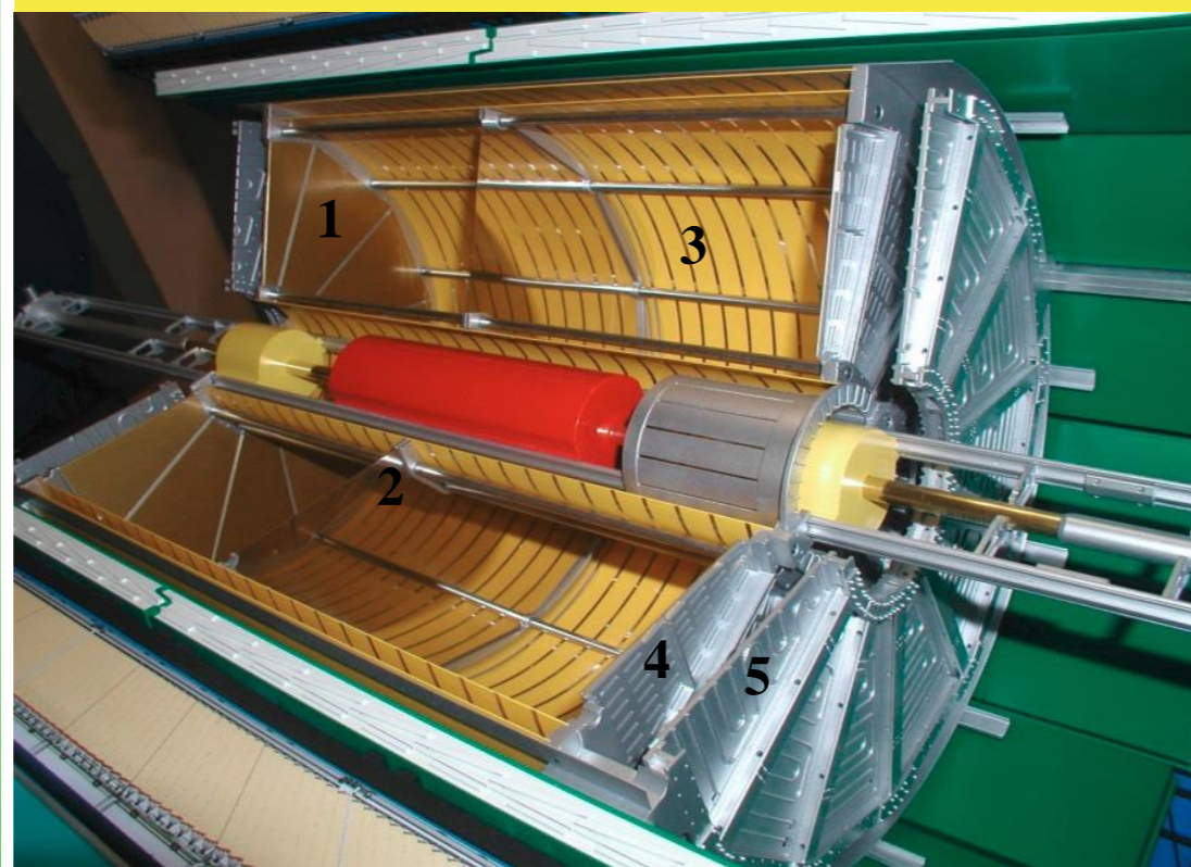
Central part of MPD mock up with TPC cross-section
