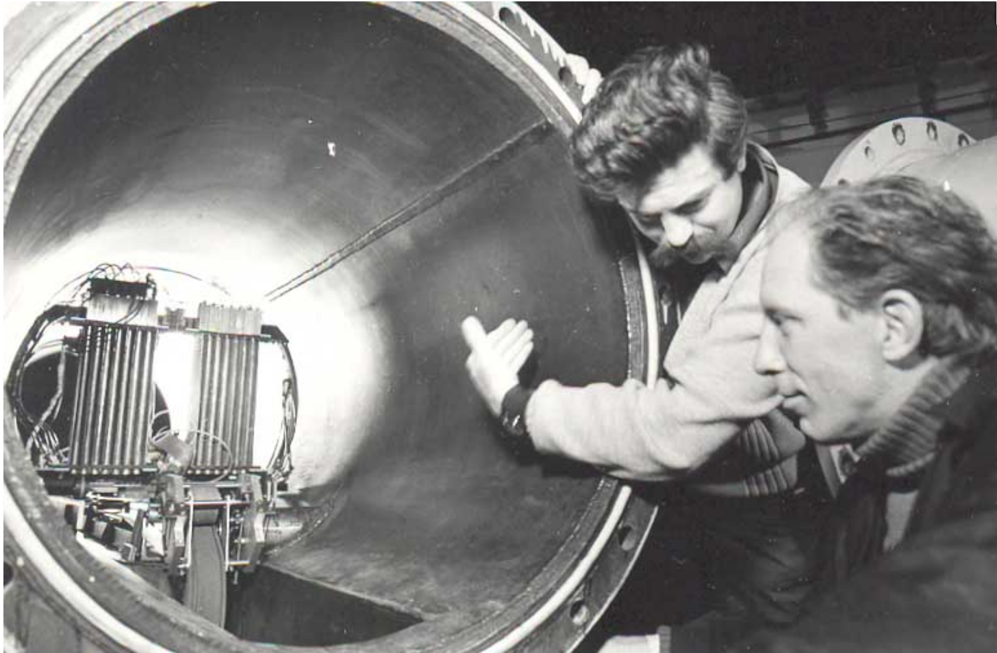
Yury Ostanevich and Laslo Cser at the first SANS detector (1974). Slit geometry, ^3\text{He} -counters inside a tube.
