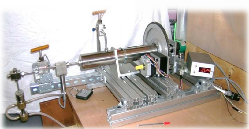
Setup for simultaneous P-V-T and SANS investigations of liquid samples
