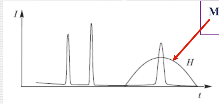
Diffraction lines and pulse of magnetic field. Dependence of diffraction intensity on field amplitude is measured.
