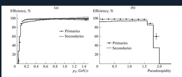
Fig. 2. Track reconstruction efficiency for particles with the number of measured points in the TPC (hits) greater than 14: (a) as a function of  $p_T$  for  $|\eta| < 1.3$ ; (b) as a function of  $|\eta|$  for  $p_T > 0.1$  GeV/c. Symbols and lines present primary and secondary particles, respectively. Secondary particles were produced within 50 cm from the interaction point.
