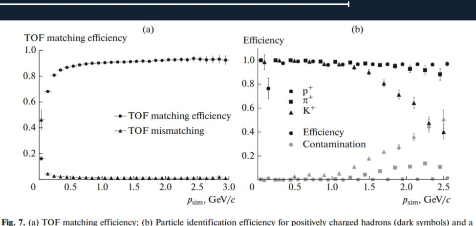
With the chosen set of cuts, charged kaons can be identified up to p=1.7 GeV/c with an approximately 80% efficiency and 20% contamination at the PID limit. Making the selection criteria for kaons tighter, the achieved contamination level can be decreased further resulting in a lower value for the PID efficiency.
