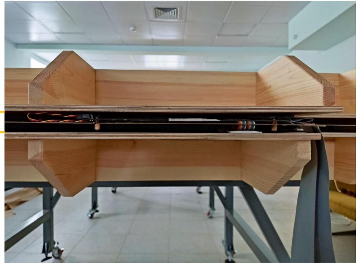
**Preliminary impression after assembly of detector plane into the slot of stand-imitator -> **30 mm gap is close to practical limit****
