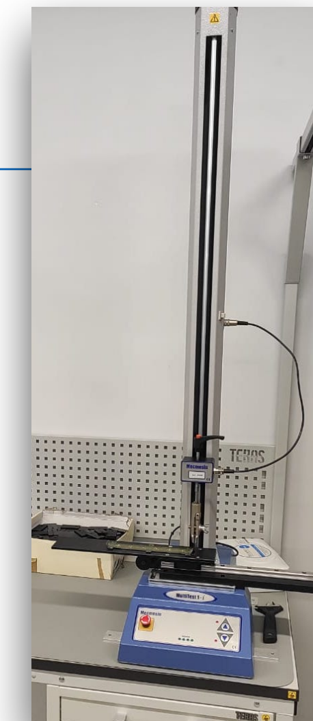
Peel test station
