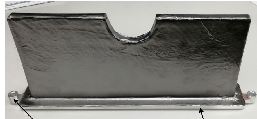
Aluminum frame of cover shielding part for Si-sensors
