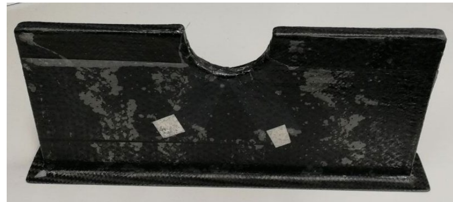
3 layers of prepreg (600 \mu\text{m} )
