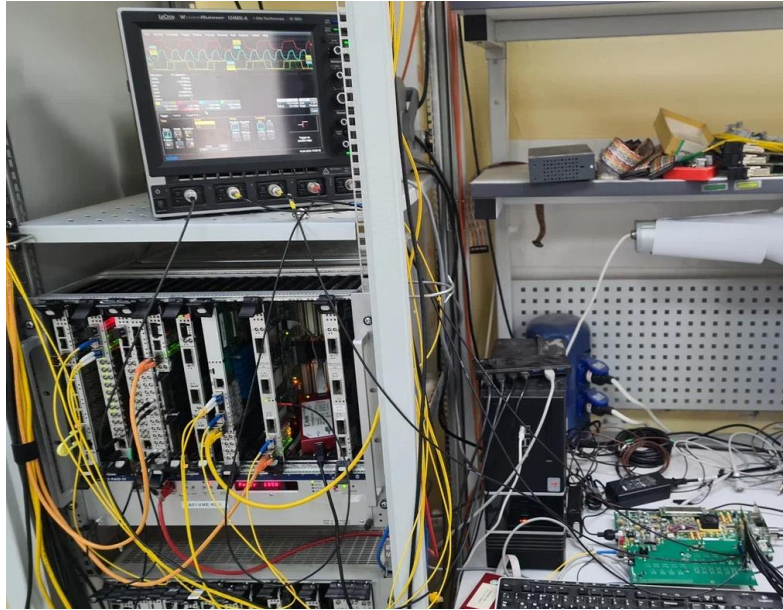
HGND readout proto_v2 connected to WR master at JINR
