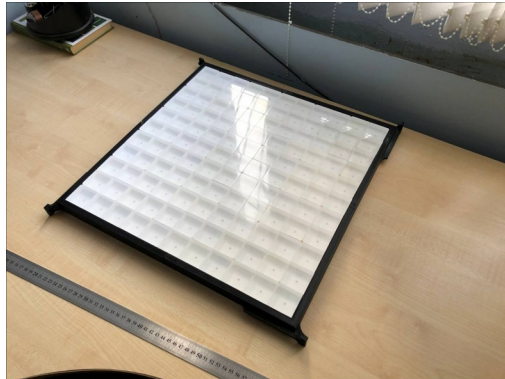
scintillator layer assembled
