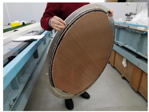
Prototypes of the calorimeter cells and SPD straw tracker endcap
